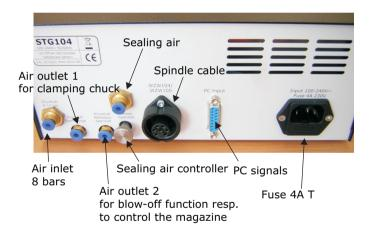
\*When using the 5-fold tool holder, please connect the air outlet 2 and the sealing air outlet by means of the Y adapter with the sealing air inlet of the spindle.
