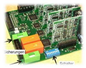
consumption or is defective. Never install fuses with higher amperage!
