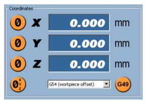
When working with several tools, it is important that the tool length compensation is switched on. Only then is the length of the current tool taken into account and added to the programmed Z value. In particular, the length compensation must also be active while you measure and set the workpiece offset (either with the height key or with the "scratch method"). Therefore, before setting up the workpiece offset, make sure that "G43" appears next to the offset by pressing the button.
