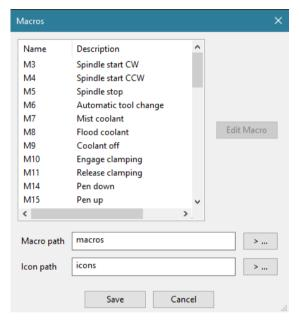
The controller can be flexibly adapted to different machines by programming so-called macros.
