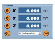
After selecting the file, it is loaded and the tool path is displayed in the graphics window. If errors are detected, the structure of the tool path is aborted at this point and a message is displayed in the lower right text window. The most common error is a "number out of range", which is usually due to a false or not yet set zero point. In this case, either select the correct zero point (G54 to G59) below the coordinate display or set a new zero point.
