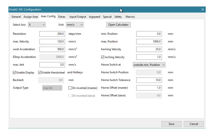
If a drive moves in the wrong direction, this can be corrected with "Inverted direction" in the axis parameters.
