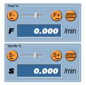
Under the spindle speed and feed controller, the current spindle speed (S) and the current feed speed (F) are also displayed. These are usually displayed in white on blue. If the option "Replace F / S global" is selected in the, these are displayed in white on turquoise.
