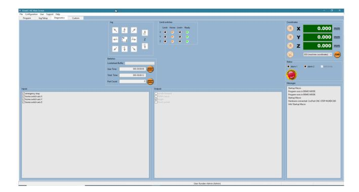
If the DEMO symbol appears instead, there is (still) no connection to the hardware. Please check this in the menu "*Configuration -> Hardware*". The symbol with the plug drawn on the far right indicates that a connection existed but was subsequently disconnected. This may not only be due to the cable connection itself but also to the operating system (anti-virus, firewall, energy-saving mode, see also chapter "*Installing the CncPOD*").
