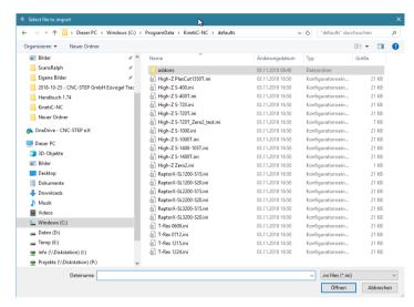
If you want to rebuild a machine, or if you want to use a fresh kit from the manufacturer, go to "Standard parameters" and select your machine. With "Standard parameters" you get to the directory of the predefined parameter sets. Attention, importing one of these files overwrites all settings made with the default values. Only do this if you want to "reset" to the factory settings and, if necessary, make a backup beforehand (see below).
