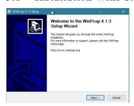
You will first be prompted to install "WinPCAP". This is a kind of universal driver software for network controllers and is required for communication of the KinetiC-NC software with the CncPod.
