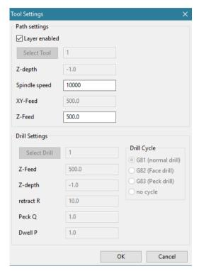
By right-clicking with the mouse on a layer in the layer list, the global settings are assigned, or you can display and modify the set values. Thus, individual values for feed, Z depth, tool or drilling can be set for each layer. The description of the individual values is identical to the global values described above.
