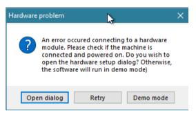
After selecting the machine model, the main window of the software opens. It is usually recommended to always turn on the machine before starting the software. If this has not already been done or there are problems with the connection, the following dialog appears:
