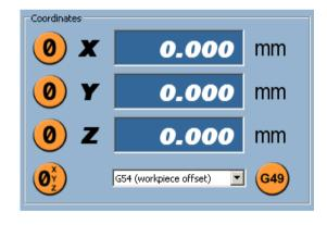
First select an offset there, e.g. "G54 (workpiece offset)". The coordinate display changes to blue background color.
