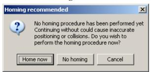
Select "Now homing" and then move to the desired position. The tip of the cutter should be just above the material surface and in the X / Y direction slightly inside the lower left corner of the material.
