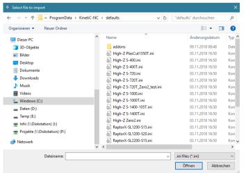
To do this, go to "File->Import settings" and select the file "HighZ\_LengthProbe.ini" in the "Addons" subdirectory under "Default parameters". This will both install the required macros and assign the input for the probe with the standard pin-assignment.
