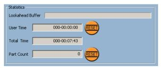
On the diagnostics page, the hours and parts counter are displayed at the bottom of Statistics. The operating hours counter and the user clock always run while a program is running.
