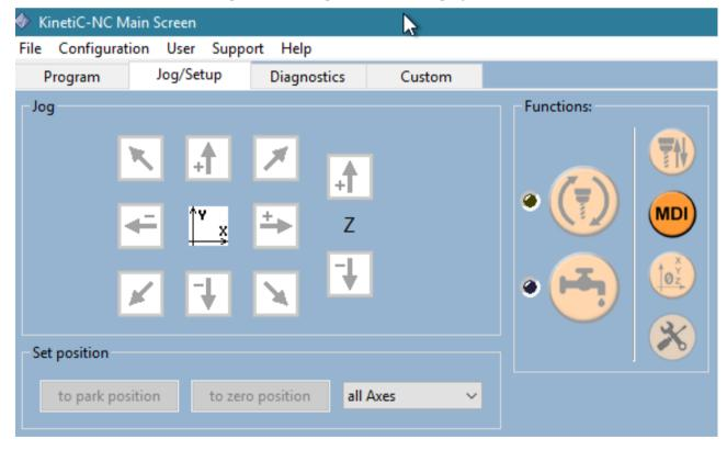
All machine movements are of course blocked as long as the emergency stop is active. Regardless of the condition of the machine, there is another reason why functions may be limited.
