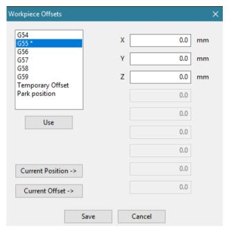
In the offset dialog, the zero offsets G54 to G59 (workpiece zero points) and the parking position are managed.
