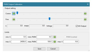
In the case of milling machines with a high-frequency spindle, the spindle speed is set using the PWM output or the laser power during laser engraving. The mapping of the S value in the NC program can be adjusted via the calibration function, it is set which minimum and maximum S value corresponds to which voltage value.
