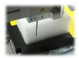
Before using for the first time, check the resolution of the C axis and the correct orientation of the knife. There are knife drives with different resolution. The tangential gauge EOT-2 has e.g. 200 full steps per revolution, which corresponds to a resolution of 5.55555 steps / ° in 1/10 micro step. The tangential EOT-3 has twice the resolution.
