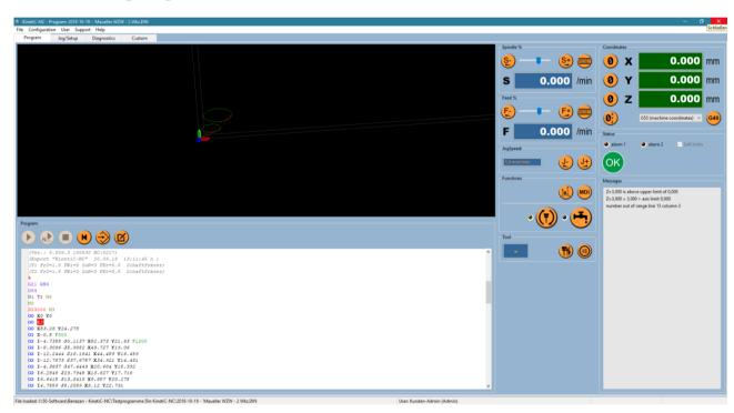
On the first page is the graphic display of the tool path, the text display of the NC program and the most important control elements to start and control the program sequence.
