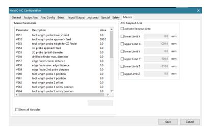
Now the height of the probe must be determined and entered into the machine parameters. First determine the approximate height of the probe with a caliper gauge and enter it in the configuration dialog on the page "Macros" at Variable number # 953 "Tool length sensor height for Z0 determination".
