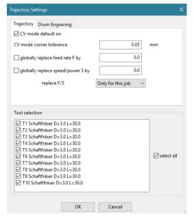
This can be useful in order to influence the path of tolerance (chord error) or feed and spindle speed afterwards, without having to change machine parameters, or having to edit the program in the text editor. If the program contains several machining steps with different tools, these are displayed below under "Tool selection". It is possible to exclude individual work steps, or to select only one of them.
