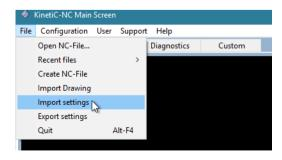
The height probe is normally connected to an extra socket on the machine or controller. For more detailed information, please refer to the documentation for your control hardware. To use the macro for hight measurement, you must first import it.
