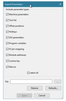
With this function you can load the complete machine parameters and all settings of the software or parts thereof from an external file. This can happen for several purposes:
