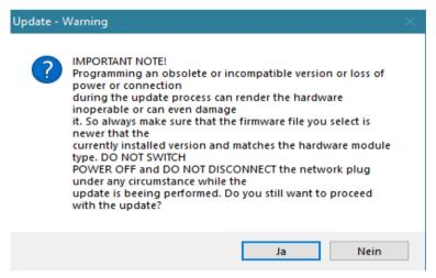
During the update, do not turn off the machine or disconnect the network cable. This could irreparably damage the module.
