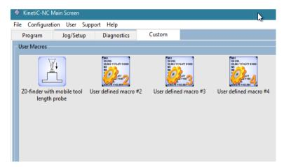
If you now remove the probe and lower it with the tool until it just touches the material, a Zero coordinate should be displayed near Zero. The small difference - ideal would be exactly zero - comes from the fact that the real switching point of the probe is located at a slightly depressed ram, and this cannot be measured accurately with the caliper.
