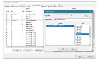
For the inputs (top right), a "tool length sensor" entry should be visible with a box to the left. In the normal state, no check mark may be displayed. Now press the button with your hand. Now a tick must be visible. If nothing changes, the probe is either not connected correctly or the signal is assigned to the wrong pin.
