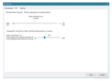
On the "Graphics" page the performance of the graphic display can be changed. For very large programs with several million line segments (depending on the performance of the PC and the graphics card from about 30MB file length) can lead to performance degradation. This is noticeable by the fact that loading takes a long time, and moving or rotating the 3D display is jerky and delayed.
