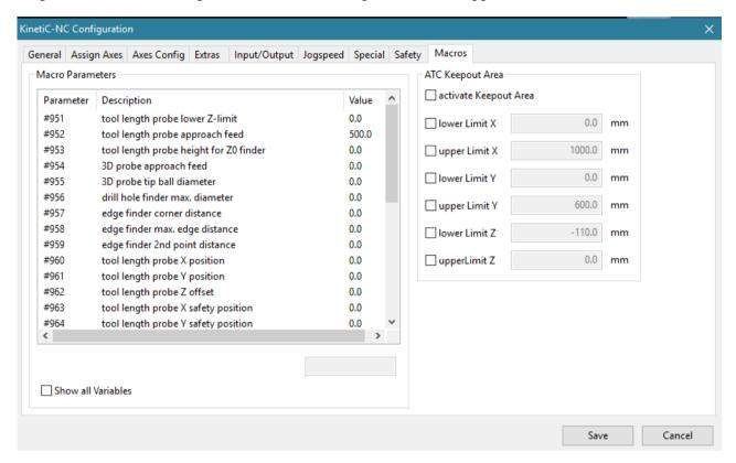
The parameters # 951, # 952 and # 960 to # 964 are used for this purpose. First enter the X and Y position where the button is mounted on the machine table. The safety position is approached after the measurement. This should be somewhere in the distance next to the button. This prevents the probe from being damaged if, after a measurement, a program is started which moves as the first movement with the Z axis all the way down.
