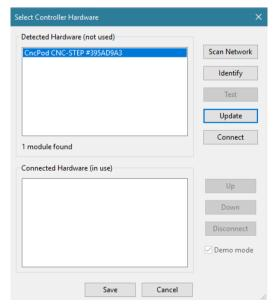
The module to be updated must be in the upper part of the list. If this is not the case, but the module is in the lower part, as in the picture on the right, select the module and then confirm the "Disconnect" button. This disconnects the machine from the software and the module is placed in the top list as unused.
