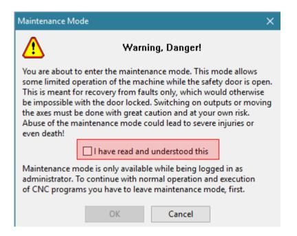
In order to prevent the maintenance mode from permanently bypassing the safety functions, the execution of CNC programs in maintenance mode is not permitted. In order to resume normal operation of the machine, maintenance mode must be exited first. This happens automatically when closing the security door.
