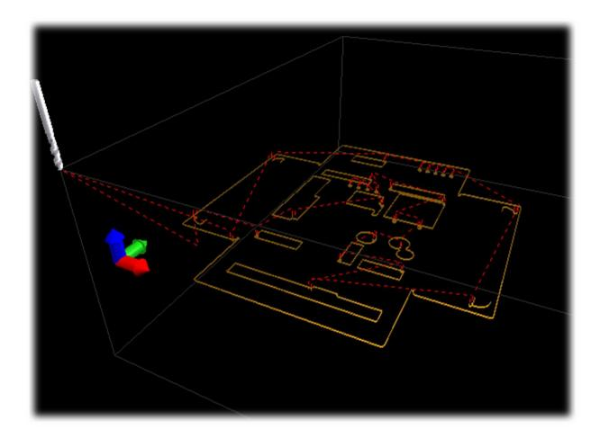
The picture above shows an example of a sheet metal part with several holes and recesses. Milling paths along the contour are normally displayed in green (possibly with different tools in other colors), rapid traverse movements with dashed red lines. The position of the zero point is represented by the three arrows in red, green and blue.
