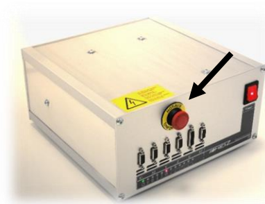
Fig. 3: Emergency-stop-button on step-motor controller
