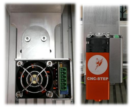
The laser connecting hub connecting CNCPOD with the laser head must be laid collision-free! Mechanical stresses on the connecting hub are to be avoided. The Hood / Door activator must be laid according to standards to ensure a conform usage of the Laser. The Laser is not operative until the Hood / Door activator is closed.
