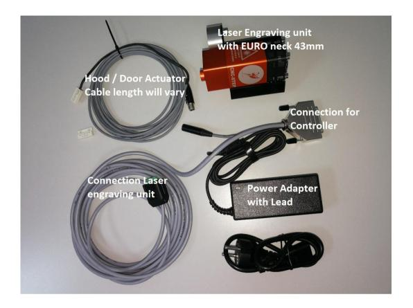
By means of appropriate measures (casing, protective barriers, suction...) it must be assured that the laser head is free of chips, dust and liquids (oil, cooling water). Metal chips and cooling water can lead to short circuits. Dust can affect the ventilation and cause overheats. Both can lead to irreparable damages and fire hazards.
