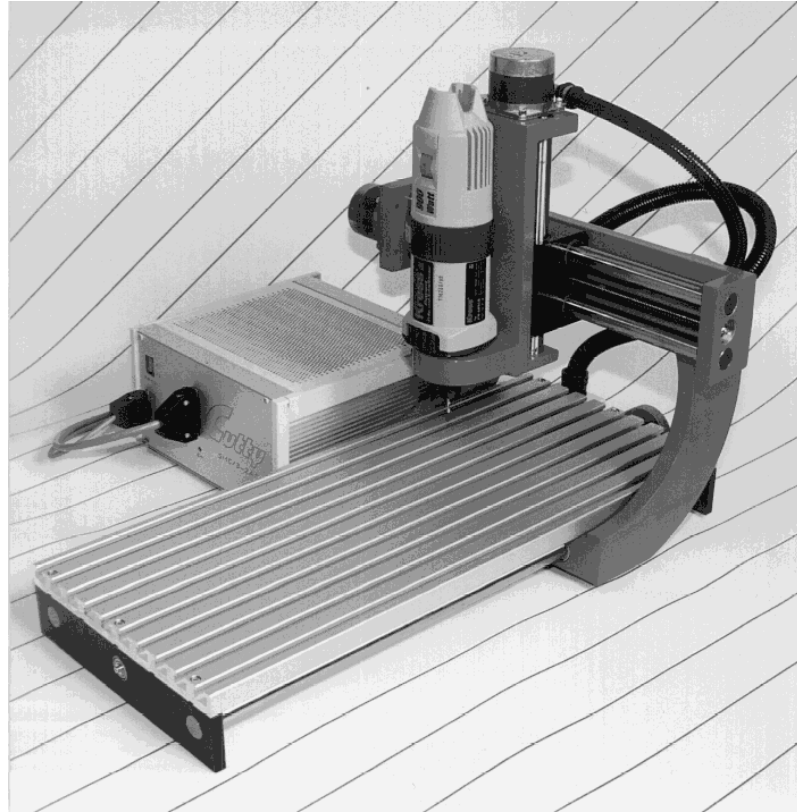
Sample of a 3 axis milling plant
